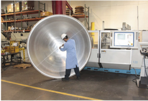
2011 photo on an 8 foot satellite dish spun at Helander. 99.38" diameter X 15.50" tall, 0.125" aluminum. +/- .060" gap on tolerance.
