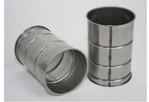
Air filtration cartridge, 26 gage 304 s/s 6.25" height X 4" i.d. Made via CNC spinning and cylinder/tube welding.
