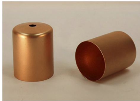
Copper float made by hydroforming 0.030" thick 2" i.d. X 4" height.
