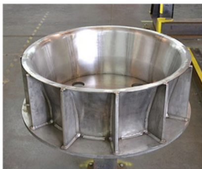
304 s/s 0.250" thick 35.00" diameter X 12.00 Height polished to a 63 Ra, spun on CNC spinning lathe.
