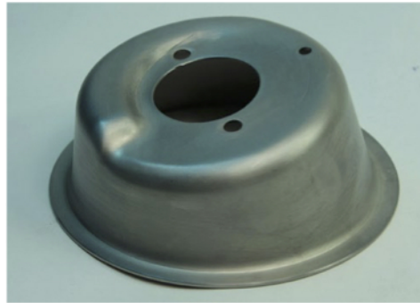
13 gauge 304 s/s spring retainer 6.5" diameter X 3.00" height made on a hydroform press.
