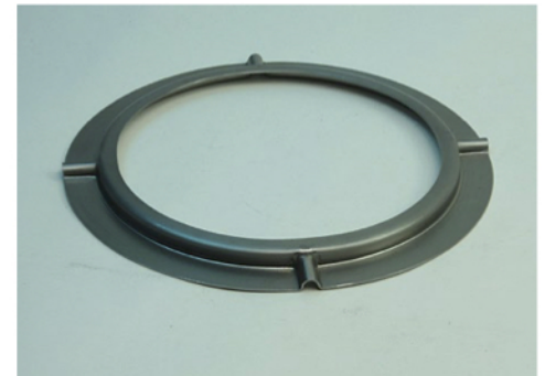
16ga 1008 steel formed using hydroforming, 9.25" diameter X 0.375" height.
