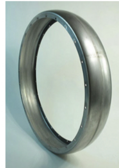
Steel ring housing used on sewer cleaning equipment. 7.00" wide X 42.00" diameter X 0.154" thick steel.
