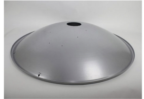
High Precision 42" diameter X 8" height 6061-0 aluminum 0.080" thick .020" RMS. Clear anodized.
