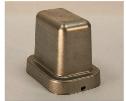
18 gage 316 s/s rectangular part, 4.10" height X 2.80" wide X 2.00" long. Part made via hydroforming.
