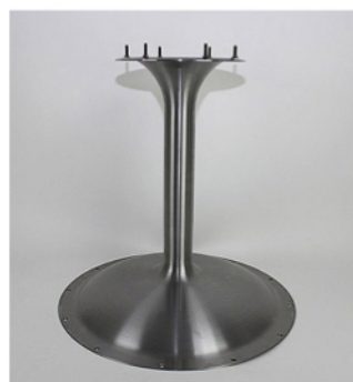
Heavy duty table column end table column, three piece welded construction polished seamless with welded studs. 25" diameter X 39" height x .075" thick steel.
