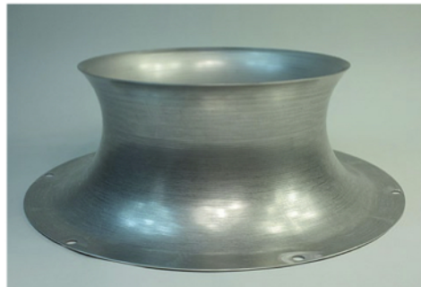
Aluminum inlet for the Commercial HVAC industry. 0.060" thick aluminum 20.00" diameter X 8.00" height formed on a CNC spinning lathe.
