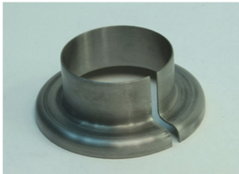
16 gauge 304 s/s, 3.00" od. X 1.50" height, formed using hydroforming.
