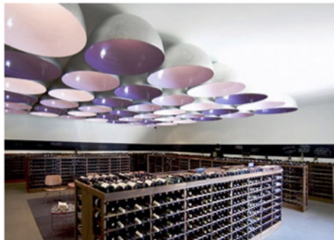
36" Hemispherical light reflectors made out of .100" thick aluminum, painted different shades of lavender for a new wine store in California.
