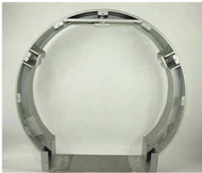
Ring housing for a medical imaging machine, 68" diameter X 20", GMAW / MIG welded, 25 pcs assembly that has been painted. Tolerances as tight as 0.020".
