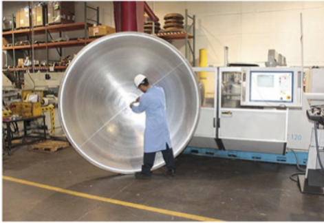
2011 photo on an 8 foot satellite dish spun at Helander. 99.38" diameter X 15.50" tall, 0.125" aluminum. +/-0.060" gap on tolerance.
