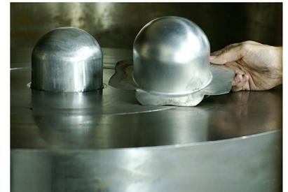
Operating at up to 10,000 psi, this hydroform features advanced control and hydraulic systems that allows us to precisely manage the forming pressure of punch travel, which facilitates the production of net-shaped parts. Its "open" feature enables our operators to visually inspect parts mid-cycle, after which they can either continue the cycle or abort in order to modify the recipe – a significant time saver in new part development projects.
