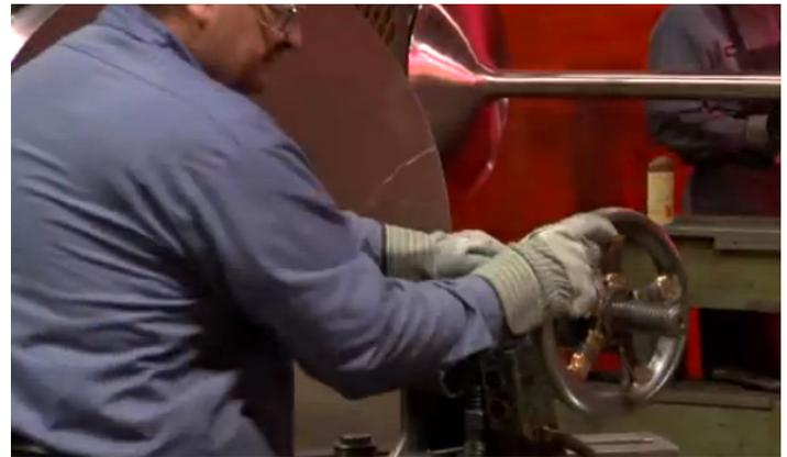
piece down the mandrel. This handle can be mounted on tool posts and use tool guides to assist the operator. The tool post acts as a fulcrum for additional leverage or a 'third hand' assisting in tool placement. For forming, the tool that is most used is called a Sheep's Nose, while a Duck's Bill is used for finishing.
