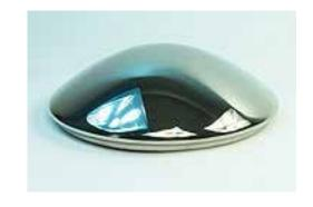
Our vintage steel hubcap is made from 16 gage stainless steel and is hydroformed in a press to achieve the shapes required for the classic car look, while still ensuring that the metal will withstand the rigors of the road. The hubcap's diameter is 10.50" and has a height of 3.125" which gives it a classic look and a highly polished finish that will withstand corrosion through everyday use.
